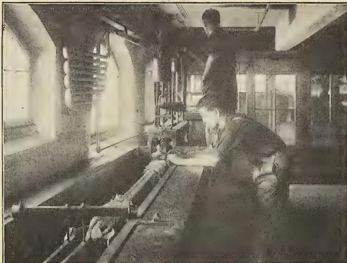
All Plymouth Rope Goes Through Rigid Inspection. A 45,000 pound pull failed to snap this 7 1/2-inch rope though it is only expected to hold 43,000 pounds.
